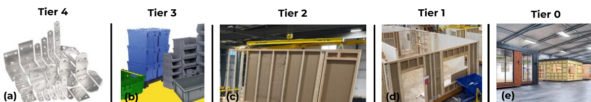
Figure 1. Multi-tiered product structure. (a) Example of items designated for consolidation into kits (Source: BREAKA brackets) (b) Representation of Kits prepared for dispatch to AC (Source: Pengoodet shop) (c) An assembled subproduct utilizing its associated kits (Source: coloradosun) (d) Representation of a volumetric
