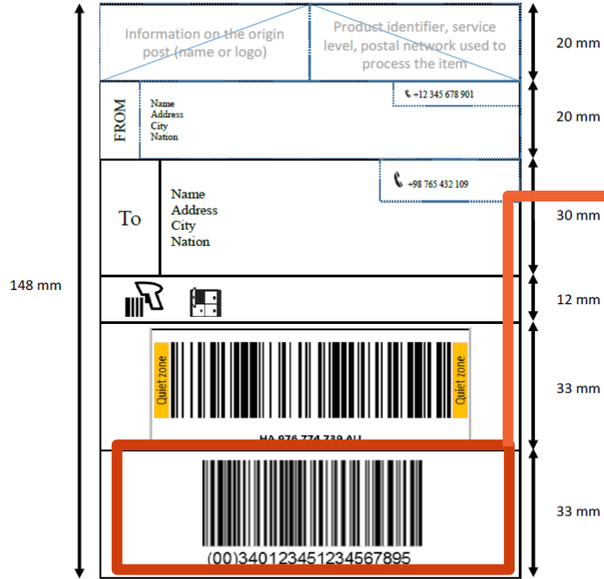
Figure 5 — Postal-item label example, including the UPU S10 and GS1 SSSC compliant standard
